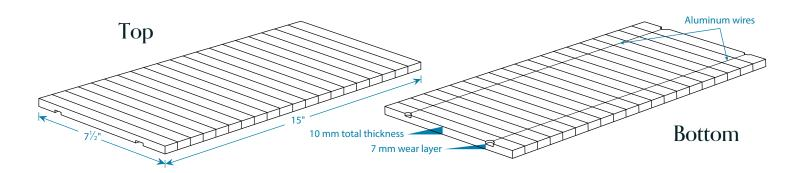
Construction: Tiles are composed of individual solid wood strips joined together by two aluminum wires. Tiles are constructed without glue to allow for seasonal movement.
